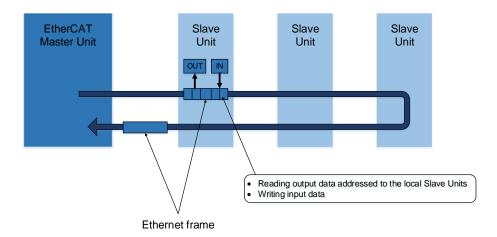
It is the "EtherCAT datagram" stored directly in an Ethernet frame that exchanges data regularly between the EtherCAT Master Unit and Slave Units.
