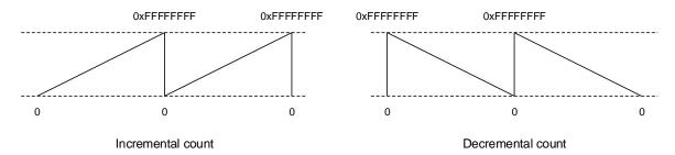
If the counter value exceeds the maximum value, the counter value returns to 0 to continue count operation. If the counter value becomes less than 0, the counter value returns to the maximum value to continue count operation.
