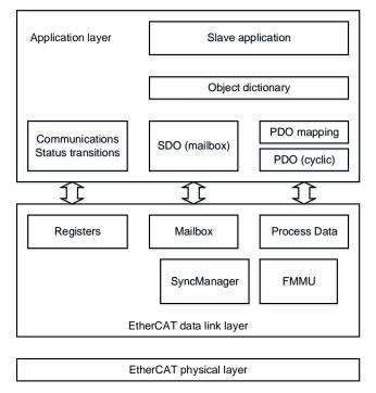
CAN application protocol has two types of object dictionaries, PDO (Process Data Object) and SDO (Service Data Object).
