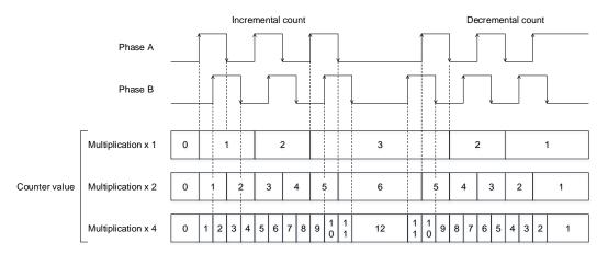
When phase A/B phase difference pulse is input, the connection with external input devices becomes as follows.
